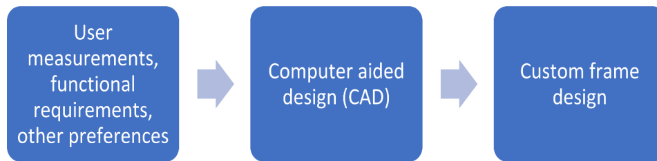
Fig. 2 Design workflow for wheelchair frame customization
